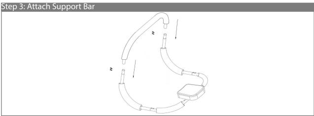
Attach Foam 950mm (2) to Support Tube (1). Secure the Support Tube using 4x M6\*10mm Bolts (5).
