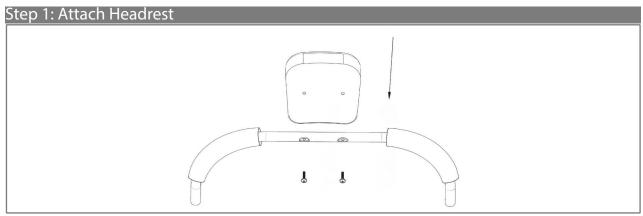
Attach the Headrest (9) to the Headrest Support (7) using 2x M6\*30mm Bolts (9).
