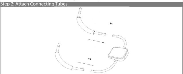
Attach 2x Connecting Tubes (4) to the Headrest Support (7). Secure this assembly with 4x M6\*10mm Bolts (5).
